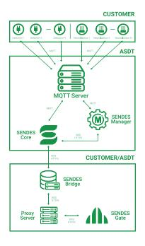
For the SENDES SJ-Box, the ecosystem enables remote (via SENDES Gate), automatic (by flight parameters), or manual activation (through the case controls, even offline).
