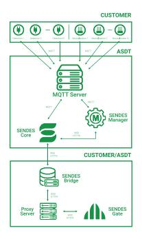
For the SENDES SJ-Box, the ecosystem enables remote (via SENDES Gate), automatic (by flight parameters), or manual activation (through the case controls, even offline).
